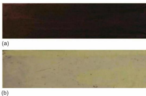
Figure 7. Surface photos of periodic WF membranes for CV dye solution treated by DCMD for 24 hours; (a) PH-E membrane and (b) PDMS-PH-E membrane
