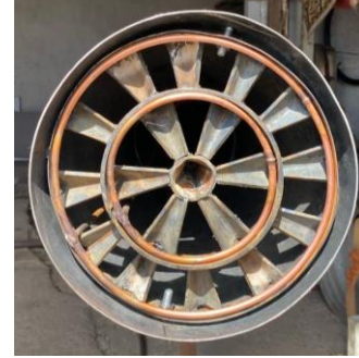
Figure 11. Front view of the burner device
