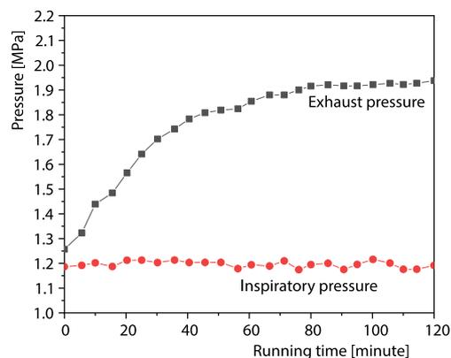
**Figure 3. Changes in exhaust pressure and suction pressure of the water thermal storage system**
