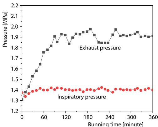
**Figure 2. Changes in exhaust pressure and suction pressure of phase change heat storage system**
