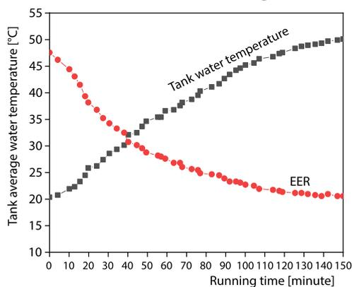
**Figure 4. Water temperature and EER variation diagram of water tank**
