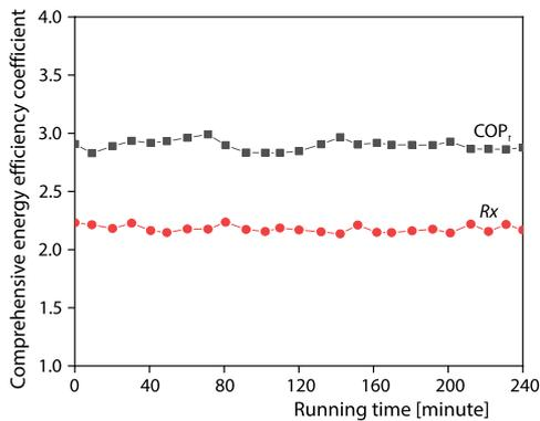
Figure 5. Change diagram of  $COP_t$  and  $R_x$  in phase change heat storage system
