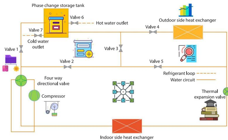
**Figure 1. Principle of phase change heat storage heat pump water heater system**
