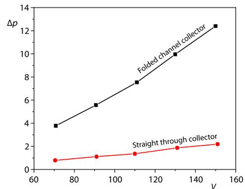
**Figure 6. Comparison of pressure drop of collectors with different structural forms**
