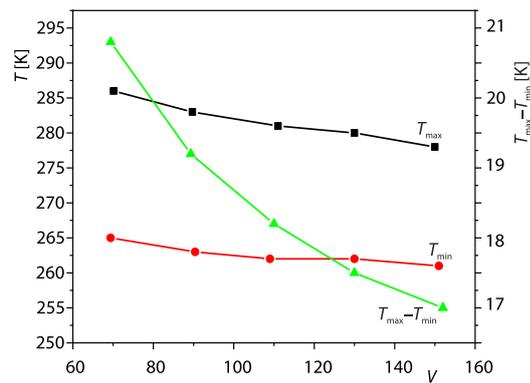
Figure 3. Effect of flow rate on the surface temperature of a collector
