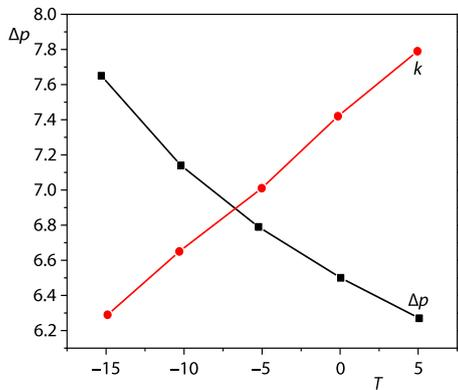
**Figure 4. Influence of inlet temperature on pressure drop and total heat transfer coefficient of collector**
