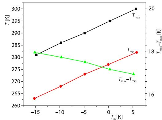
**Figure 5. Effect of inlet temperature on the surface temperature of a collector**
