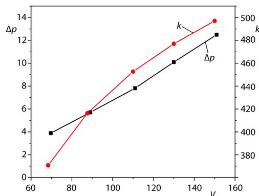
Figure 2. Effect of flow rate on pressure drop and total heat transfer coefficient of collector
