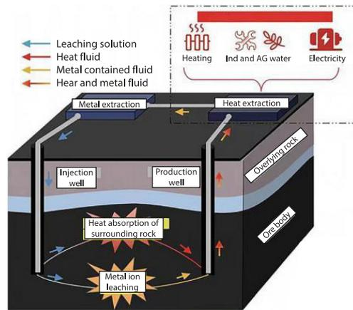
**Figure 2. Schematic diagram of enhanced geothermal co-mining process for fluidized bed leaching of metal ore**
