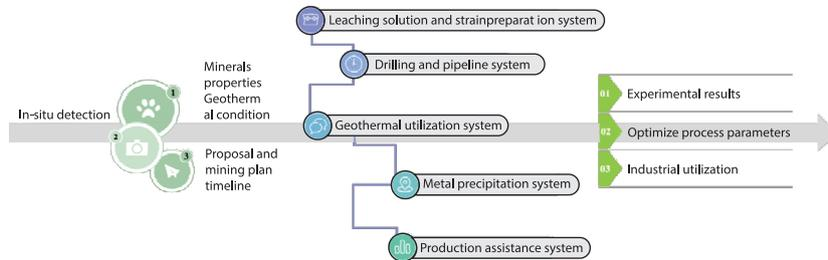
**Figure 1. Flow chart of enhanced geothermal collaborative co-mining process for fluidized leaching of deep ground metal mines**
