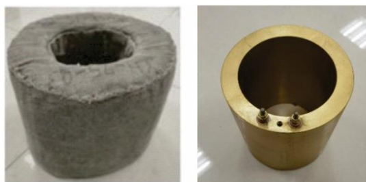
Figure 10. Thermal insulation material testing unit with metal heater
