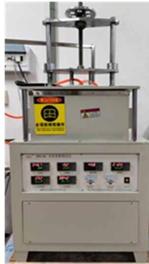
Fig.4 DRS-3A high-temperature thermal conductivity meter
