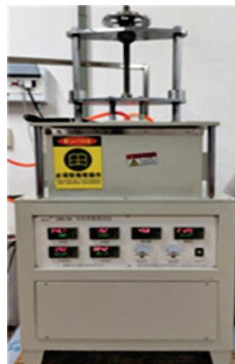
Figure 4. The DRS-3A high temperature thermal conductivity meter
