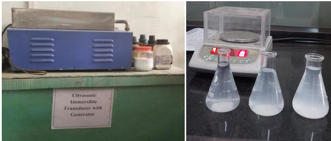
Figure.3. Ultrasonic immersible transducer with generator and samples of nanolubricant
