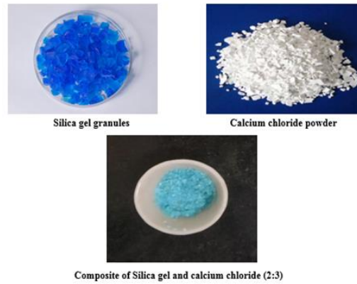
Fig.1. Preparation of desiccant material
