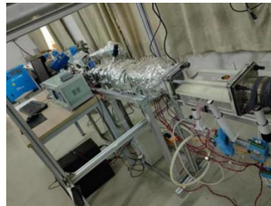
Figure 2. Photo of experimental system wrapped with insulation cotton
