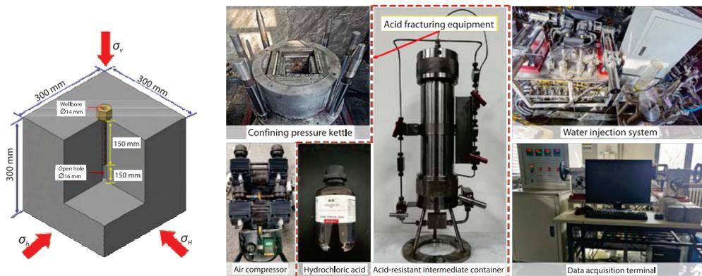
**Figure 1. Experimental material and true triaxial acidizing fracturing equipment**
