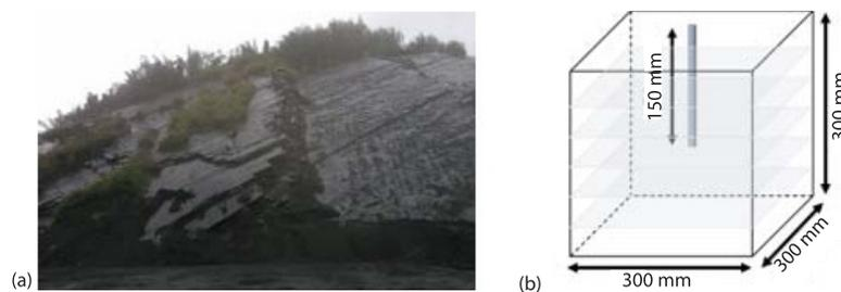
Figure 1. Outcrop collection (a) and specimen processing (b)
