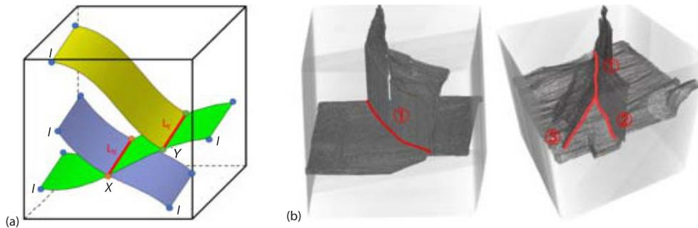
Figure 5. Schematic diagram of crack intersecting lines (a) and the red line is the intersecting line in the 3-D crack map (b)
