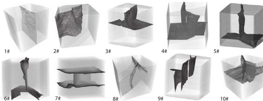
**Figure 2. The 3-D reconstructed structure of cracks in 10 sets of specimens**
