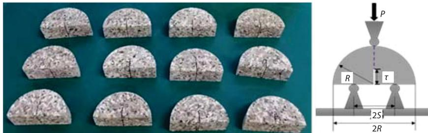
Figure 1. Granite specimens and their experimental loading schematic diagram
