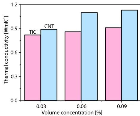
**Figure 4. Thermal conductivity of TiC and CNT nanofluid**
