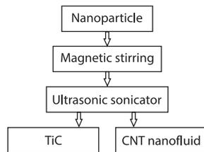
**Figure 3. Nanofluid preparation**
