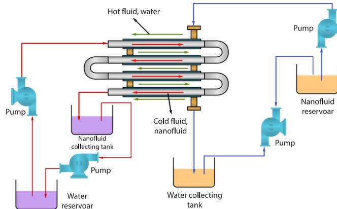
Figure 2. Systemic flow diagram of a counterflow DPHE
