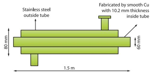
Figure 1. Specifications of twin pipe heat exchanger
