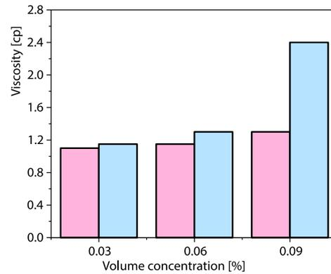
**Figure 5. Viscosity of TiC and CNT nanofluid**
