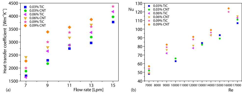
Figure 6. (a) Heat transfer coefficient and (b) Nusselt number during tests with the flow of TiC and CNT nanofluids
