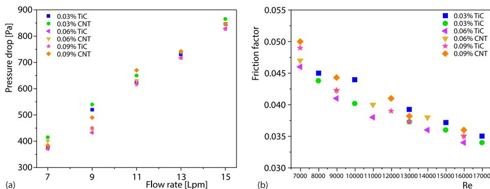
Figure 7. (a) Coefficient of friction using the Reynold’s number and (b) flow rate using pressure dropsthe of TiC and CNT nanofluids
