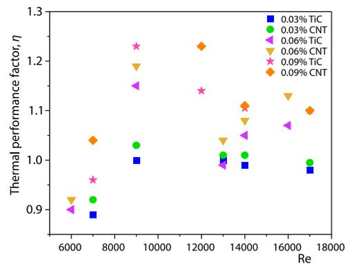
Figure 8. Thermal performance factors of the TiC and CNT nanofluids
