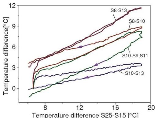
**Figure 4. Comparison of temperature variation and rise over solar chimney temperature**
