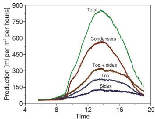
**Figure 3. Distillation productivity rate (solar still chimney)**
