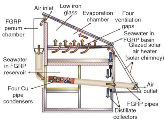
**Figure 1. Diagrammatic cross-section of a solar still with chimney and solar still with the condenser**
