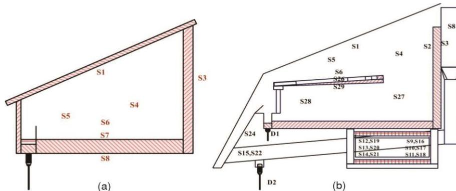
**Figure 2. Comparison of standalone solar still thermo-couples; (a) without and (b) with chimney**
