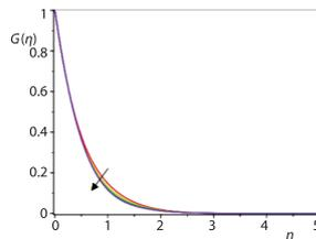
Figure 15. Effect of  $Nt$  on velocity profile
