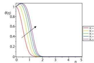
Figure 16. Effect of  $Nt$  on temperature profile
