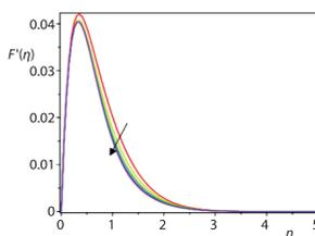
Figure 14. Effect of  $Nt$  on velocity profile
