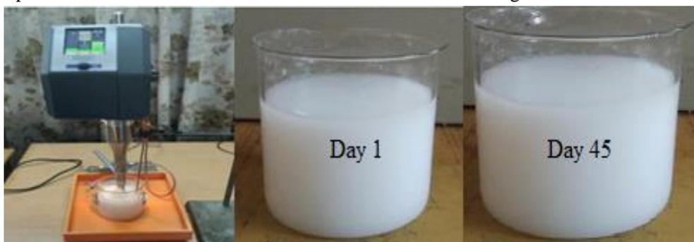
Figure 1. Preparation and stability testing of  $\text{Al}_2\text{O}_3$ -deionized water nanofluid
