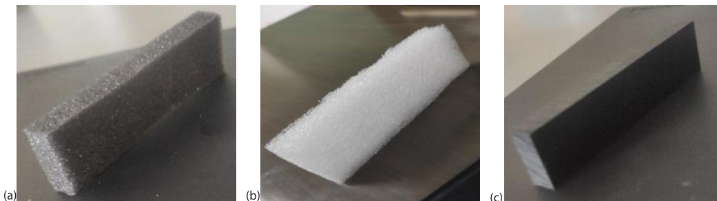
Figure 1. Structure materials; (a) polyurethane sponge, (b) EPE pearl foam, and (c) carbon fiber board
