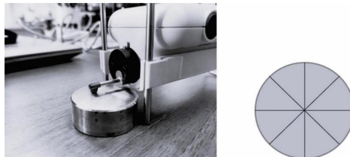
Figure 4. Surface roughness measurement and schematic representation of the measurement paths
