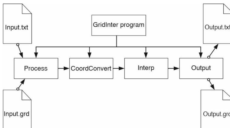
Figure 3 Diagram of the GridInter terrain grid program
