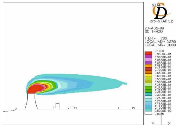
Figure 16. The NNW wind direction cooling tower heat plume cross-sectional concentration distribution
