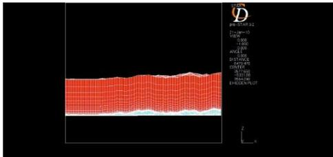
Figure 12. Side view of fluid body mesh
