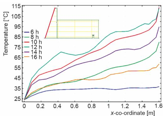
**Figure 4. Temperature evolution at the outside glazing**
