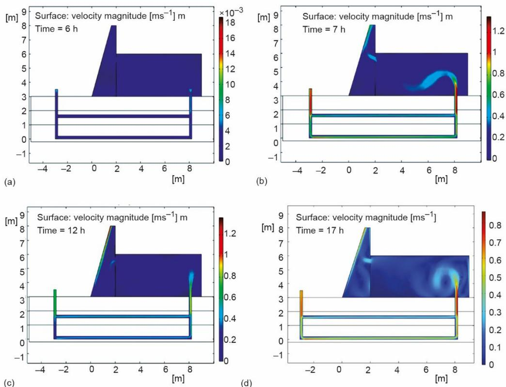
**Figure 10.** Air velocity distribution within the room and the underlying soil during peak hours, specifically at; (a) 6 a. m., (b) 7 a. m., (c) 12 p. m., and (d) 5 p. m.
