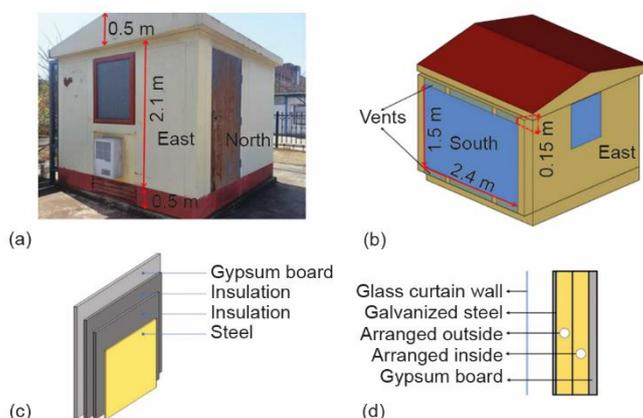
**Figure 1. An exemplification of an experimental building situated in Changsha, a region characterized by a hot summer and cold winter climate in China [5]; (a) experimental lightweight building, (b) retrofit building with Trombe wall, (c) conventional building envelope, and (d) Trombe wall building envelope**
