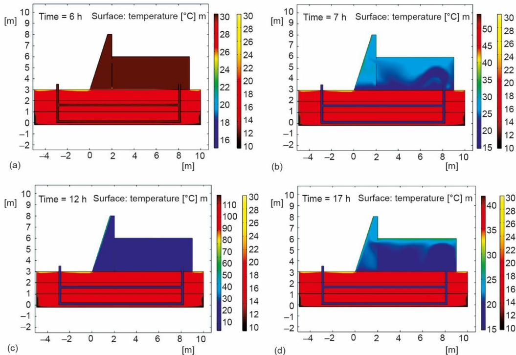
**Figure 9.** Temperature distribution within the room and the underlying soil during peak hours, specifically at; (a) 6 a. m., (b) 7 a. m., (c) 12 p. m., and (d) 5 p. m.
