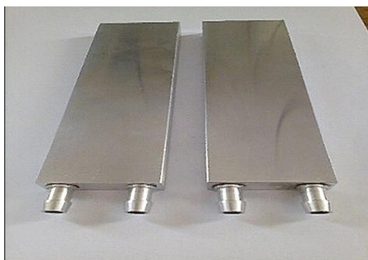
Figure 3. Aluminum heat exchangers utilized in the experiment
