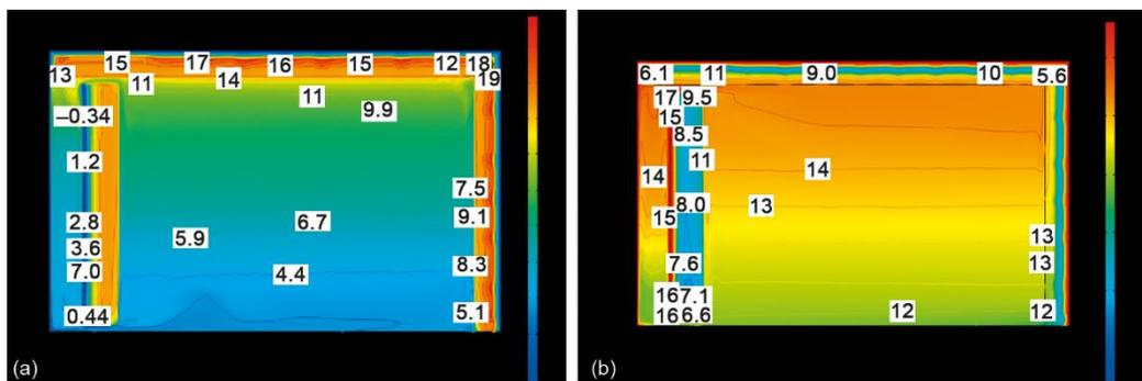
Figure 6. The indoor isotherm at two distinct time points; (a) 02:00 h and (b) 08:00 h
