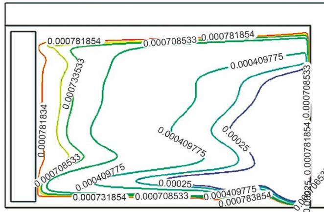
**Figure 8. Spatial distribution of air inlet and outlet velocities within the enclosure**
