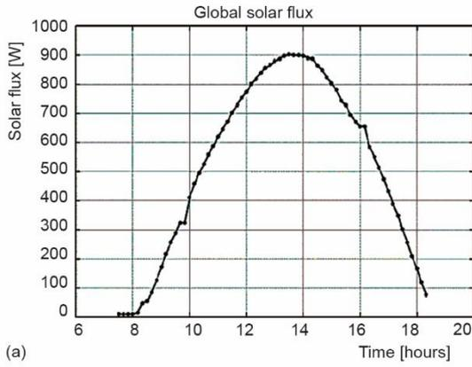
Figure 3. Winter solar flux incident on the glazed wall
