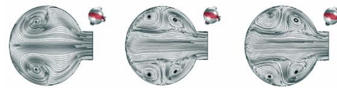
Figure 5. Distribution of the flow fields on the vertical plane; (a) Re = 100, (b) Re = 2000, and (c) Re = 2500
