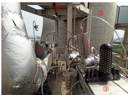
Figure 1. Experimental test platform; ① horizontal flue, ② chimney, ③ enamel condensing heat exchanger, ④ ELPI
