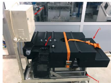
Figure 5. Testing equipment; 1 – speedometer instrument panel, 2 – fuel level measurement sensor, 3 – fuel tank, and 4 – slide mechanism
