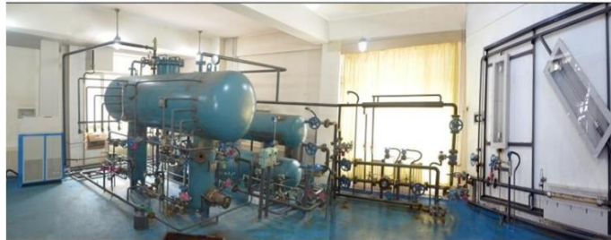
Figure 5. The main circulation system of the test bench
