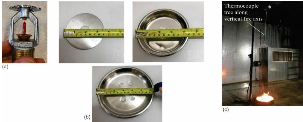
Figure 2. Experimental devices; (a) sprinkler heads, (b) HCP: HCP-A: 90 mm diameter, HCP-B: 110 mm diameter, HCP-C: 165 mm diameter, and (c) fire chamber test
