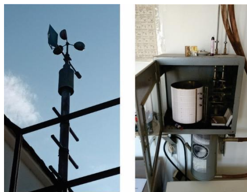
Figure 1. Photograph of instrument that is used for measurement of wind speed
