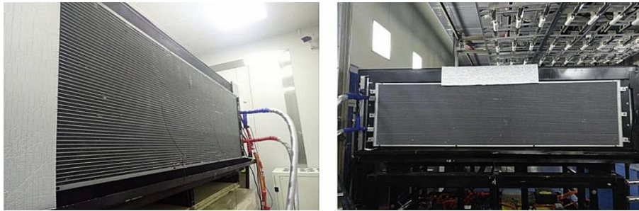
Figure 4. Parallel flow heat exchanger inside and outside the vehicle
