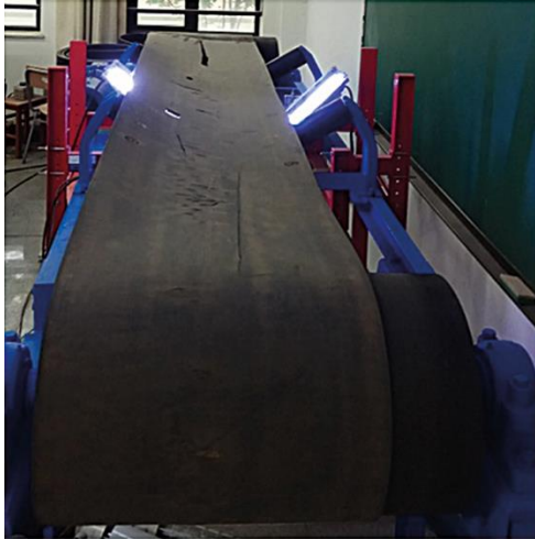
Figure 4. Deviation fault test
