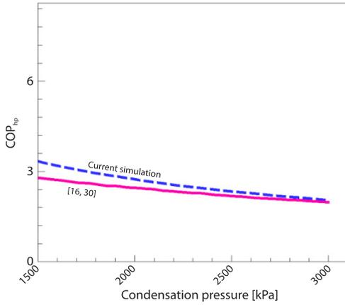
**Figure 3. Comparison of the results of the present work with the results of [16, 30]; the effect of condensation pressure changes on the heat pump coefficient of performance**
