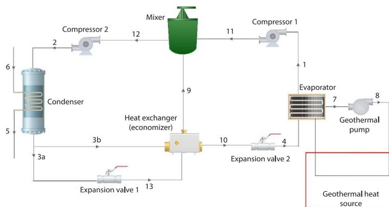
Figure 1. Cycle of the geothermal heat pump, shown schematically
