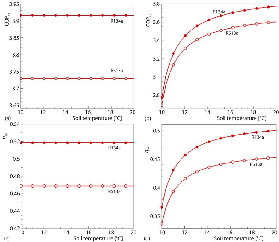
**Figure 5. Changes in (a)  $COP_{hp}$ , (b)  $COP_{tot}$ , (c) heat pump exergy efficiency, and (d) total exergy efficiency relative to soil temperature changes for the working fluids under study**
