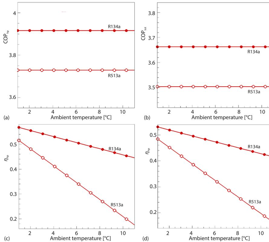
**Figure 4. Changes in (a)  $COP_{hp}$ , (b)  $COP_{tot}$ , (c) heat pump exergy efficiency, and (d) total exergy efficiency relative to ambient temperature changes for the working fluids under study**
