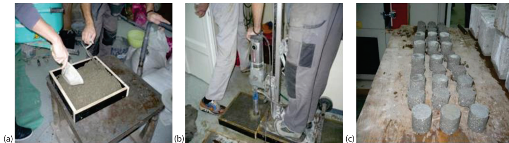
Figure 1. Pouring the mortar mixture (a), extracting cylinders from molds (b), and (c) appearance of the specimens
