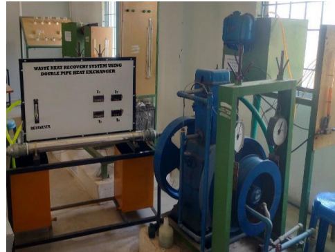
Figure 1. Experiment set-up of PFDPHE for waste heat recovery system
