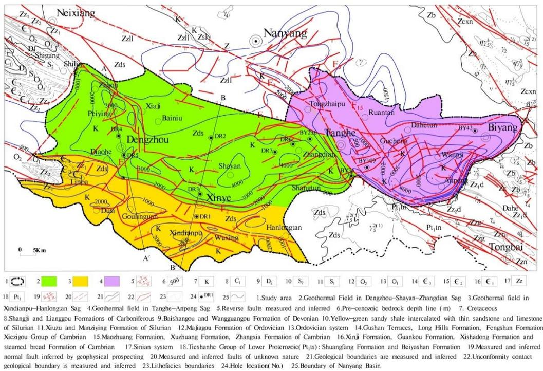
Figure 1. Geological Structure and Geothermal Field Zoning Sketch Map of Nanyang Basin
