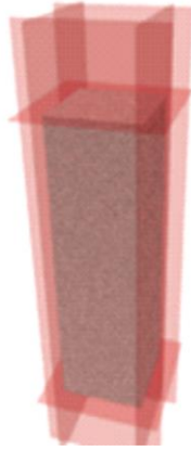
Figure 1. The PFC rock model and boundary conditions
