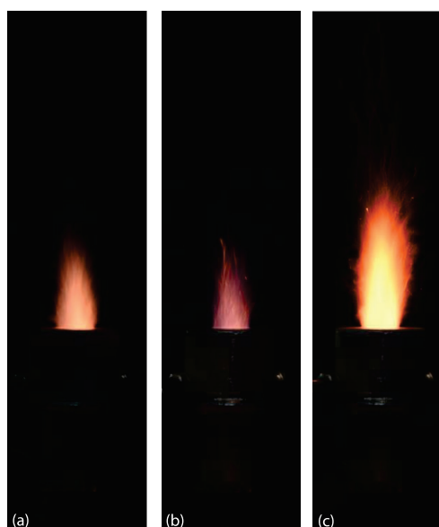
Figure 3. Typical photos of the flame in various combustion regimes; (a) combustion of diesel fuel without secondary air and coal: F_v = 0.58 kg per hour, F_f = 0.7 kg per hour, (b) combustion of diesel fuel with secondary air without coal: F_v = 0.57 kg per hour, F_f = 0.7 kg per hour, F_{a2} = 4 kg per hour, and (c) co-combustion of diesel fuel and pulverized coal: F_v = 0.59 kg per hour, F_f = 0.7 kg per hour, F_c = 0.1 kg per hour, F_{a2} = 4 kg per hour
