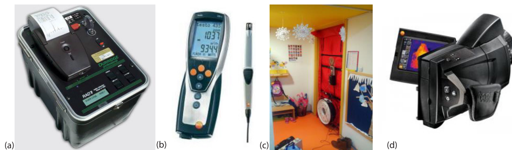
Figure 3. Devices used for measurement: RAD 7 (a), Testo 435-2 (b), Minneapolis Blower Door (c), and Testo 885-2 (d)
