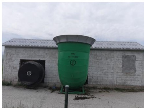
Figure 3. Depiction of Štavalj mine main (AVJ-1500) and spare (N-AVV-D) fans
