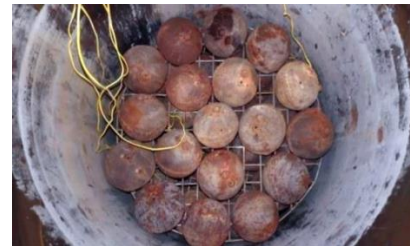
Figure 5. Arrangement of PCM capsules in the TES tank
