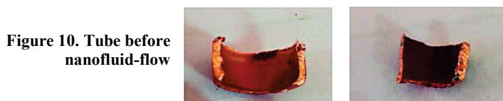
Figure 11. Tube after nanofluid-flow
