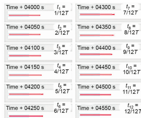
Figure 8. Iso-surface of vapor volume fraction equals 0.97
