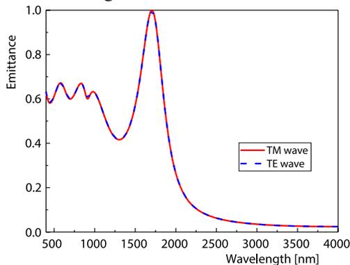
**Figure 5. Emittance spectrum in TM and TE polarization modes**
