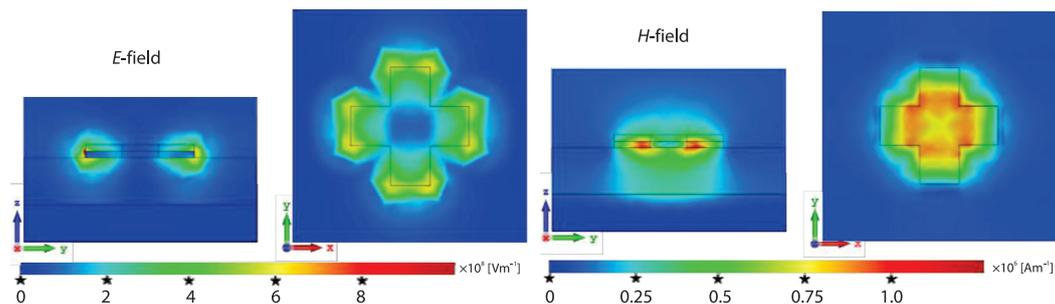
Figure 7. Electric field,  $|E|$ , and magnetic field,  $|H|$ , distribution of selective emitter at wavelength of 1700 nm
