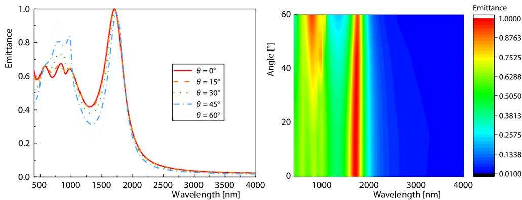
Figure 6. Emission spectrum and 3-D distribution of emitter under different incidence angles
