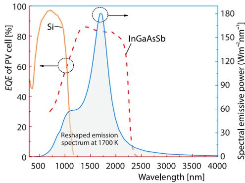
**Figure 3. The EQE curve of Si and InGaAsSb PV cells and reshaped emission spectrum by selective narrowband emitter**
