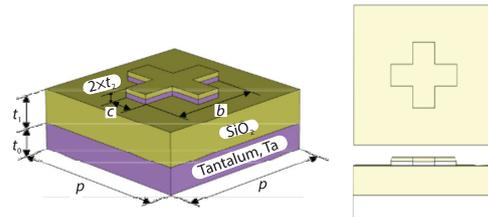
Figure 2. The geometry and structural parameters of selective emitter
