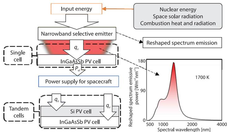
Figure 1. Schematic for system energy conversion process
