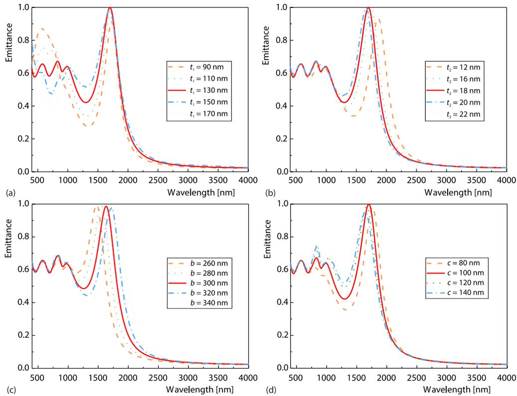
**Figure 4. Variation of selective emitter emittance with; (a) thickness  $t_1$  of the second dielectric  $\text{SiO}_2$  layer, (b) thickness  $t_2$  of the third and the fourth cross patch layers, (c) length  $b$  of cross patch, and (d) width  $c$  of cross patch**
