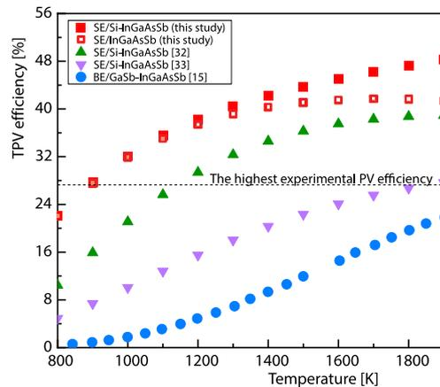
Figure 8. Comparison of the different TPV systems efficiency with temperature
