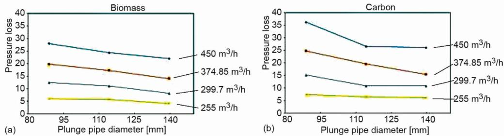
**Figure 11. Biomass and coal pressure loss**
