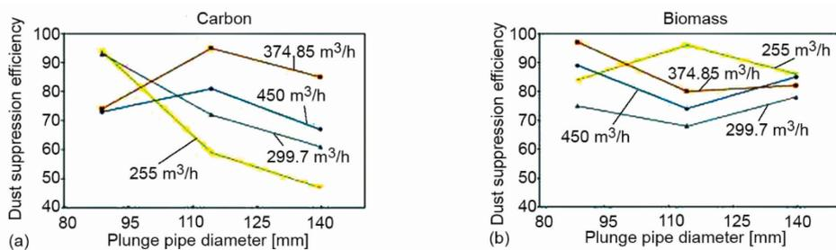
Figure 10. Biomass and coal dust suppression efficiency in experimental study
