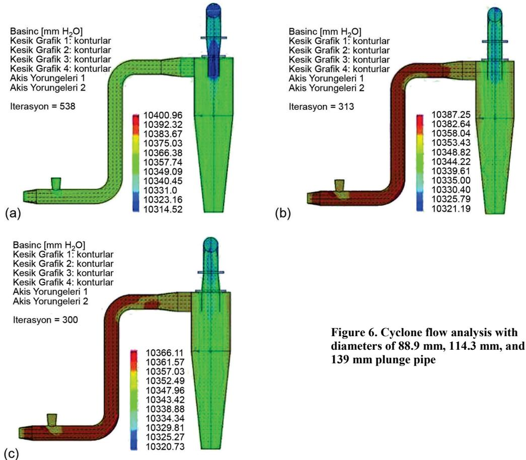
Figure 6. Cyclone flow analysis with diameters of 88.9 mm, 114.3 mm, and 139 mm plunge pipe
