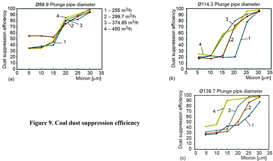
Figure 9. Coal dust suppression efficiency
