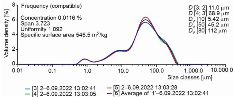
Figure 12. Biomass Mastersizer 3000 laser solid particle analysis
