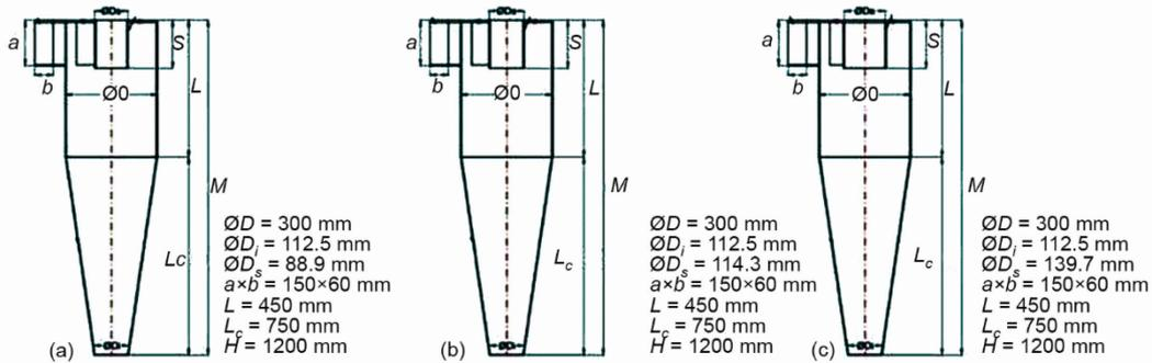
Figure 5. Cyclone plunge pipe diameter features
