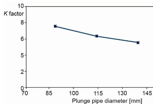
Figure 14. Pressure loss factor calculation
