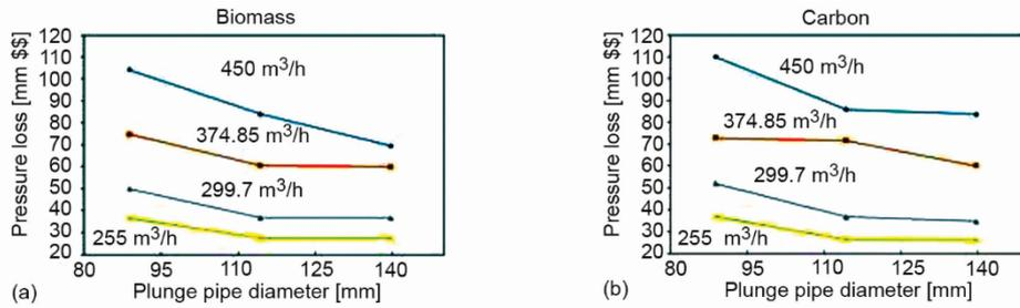
Figure 7. Biomass and coal pressure loss diameter [mmSS]
