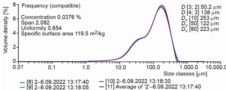
Figure 13. Coal Mastersizer 3000 Laser solid particle analysis
