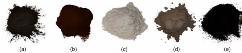
Figure 1. Dust samples; (a) cement, (b) bricks, (c) white cement, (d) fly ash, and (e) coal
