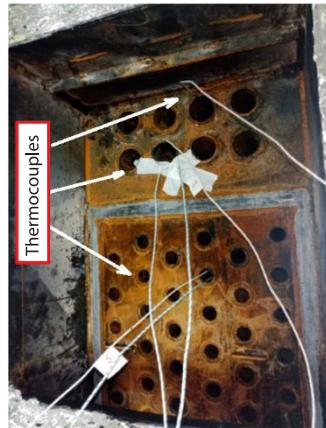
**Figure 5. Mounted TC in pipe heat exchanger of hot air generator**
