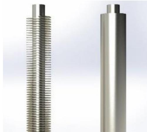
**Figure 11. Real geometry of a heat exchanger inside hot air generator and a porous geometry with equivalent characteristics**
