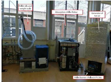
**Figure 1. Laboratory of MEF Niš with Pellet Silo on the left, absorption heat pump in the middle and hot air generator on the right with pellet burner**
