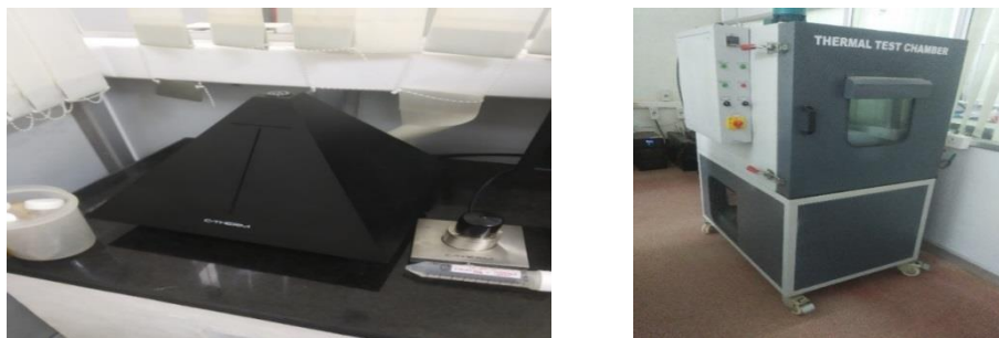
Figure 6. (a) C-Therm TC analyser and (b) thermal test chamber
