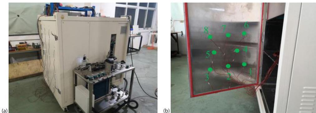
**Figure 4. Validation platform; (a) RCTB and (b) arrangement of measurement points**
