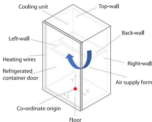
**Figure 1. Refrigerated container (3-D view)**
