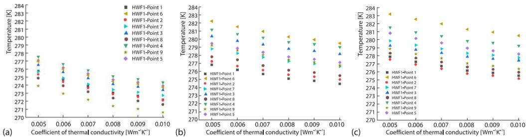
**Figure 9. Temperature of nine points with different thermal conductivity; (a) HFW1, (b) HFW2, and (c) HFW3**
