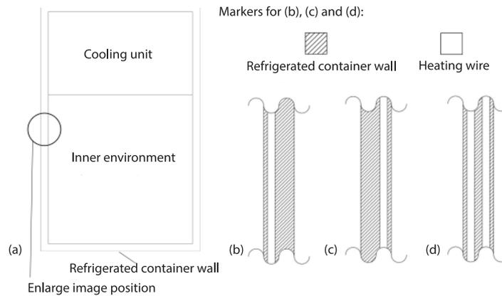
**Figure 2. Heating wire forms; (a) enlarge image position for (b)-(d) (front view, cross-section), (b) HWF1 (enlarge image), (c) HWF2 (enlarge image), and (d) HWF3 (enlarge image)**
