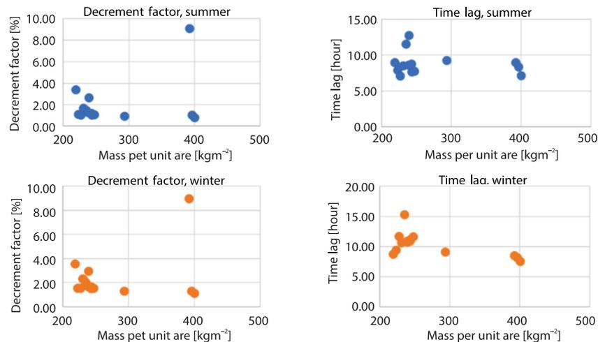
**Figure 4. Decrement factor (left) and time lag (right) vs. mass per unit area for 14 clay block structures for summer (upper) and winter (lower) conditions**
