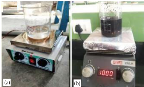
Figure 2. Preparation of composite phase change material; (a) pure paraffin wax and (b) graphite powder with paraffin wax
