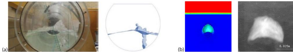
Figure 1. Verification of mathematical model; (a) verification of multi-lance for bottom blowing [32] and (b) verification of single lance model for bottom blowing [34]
